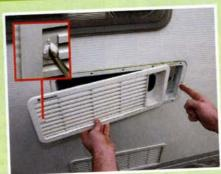
The main vent cover is detached after turning the turn-buckle anti-clockwise (inset) then lifting away from the left. When refitting, push the slotted hole on to the long peg.
