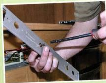
The fridge front trim panel, removed earlier, should be covered in masking tape, carefully measured and marked out, centre punched, drilled and the new switch screwed carefully into place.
