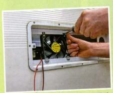
The 'Meccano-style' strips supplied were cut down to fit the fan to the aluminium deflector with self-tapping screws while the lower part, bolted to the plastic, was reinforced with washers.
