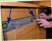
Inside the caravan, you need to access the Dometic fridge top. Pull off the three knobs, unscrew the catch and then remove the two screws (arrowed) to remove the cover.
