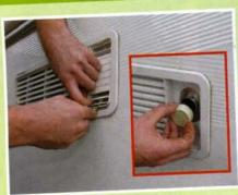
On a standard Dometic caravan fridge vent, you push the tag down with a screwdriver and lift off the exhaust trim then unclip the oval pipe cover from underneath (inset).
