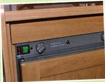
The switch allows OFF, permanent running or thermostat. Then, the built-in air temperature sensor switches on the fan automatically when the temperature behind the fridge reaches 30 to 35°C.
