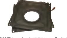
VW T4 swivel 1997 on. Bolt holes on seat box. 426 x 404mm
