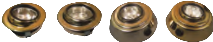
L9067 Recessed swivel 10w halogen spot (0.83 amps) (no switch) cut out hole diameter 55mm minimum x 22 deep, outer bezel 70mm. 12 Volt L9067C Recessed spot (chrome). L9067D Recessed spot (gold) L9067MN Recessed spot (matt nickel).
