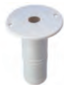
HFS4504 Long tail hole tidy/floor seal. 8-15mm Pipe Seal 75mm Tail. Fits snug in 24-25mm hole. Colour Off White
