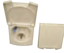
Mains inlet socket styled to match F30/1 water filler (page 17). Sizes 137mm High x 122mm Wide. Cut out oval 90mm H x 85mm W. MIF30 White mains inlet MIF31 Black mains inlet
