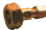
GT120 Tank connector for remote gas regulator (GT2005-2) with 1/2" left hand female thread inlet & 8mm olive outlet for copper pipe.
