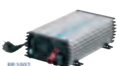
DPP1002 - 12v DC Modified sine wave inverter. Continuous power 1000W Peak power 2000W (WxHxDmm) 176 x 95 x 338
