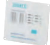
DMCR7 Low-voltage, over-voltage, Power on indicated by red LED overheat and overload indicated by red LED's, stand-by and power on indicated by green LED's. 7.5mtr connection cable. For use with : DMSP702 - DMSP2512
