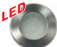
NEW LED30FSRMN LED Fixed recessed or surface mount with surround supplied. Led downlight of superb quality with 30 LED's for high output. Connect to 12volt DC. 1.8w Size 70mm Ø x 17mm recessed or 32mm High surface mounted.
