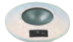
Mini Halogen down lighter 10w 12v. Sizes OD 80mm, installed height 10mm (cut out 60mm dia x 15mm deep). L1009W WHITE NO SWITCH L1009SW WHITE WITH SWITCH
