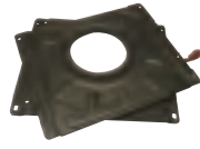
SWVL3R Boxer, Ducato, Relay, RH drivers 1994 to 2006 model year. SWVL3L Boxer, Ducato, Relay, LH passenger 1994 to 2006 model year. Re-use seat belt mounting on seat 430 x 350mm (3R pictured) FASP
