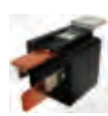
R228 Relay 70A for linking batteries for split charging & running fridge 12V feed from engine.
