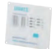
DMCR7 Low-voltage, over-voltage, Power on indicated by red LED overheat and overload indicated by red LED's, stand-by and power on indicated by green LED's. 7.5mtr connection cable. For use with : DMSP702 - DMSP2512
