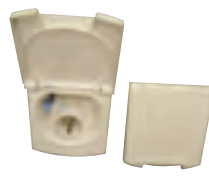
Mains inlet socket styled to match F30/1 water filler (page 17). Sizes 137mm High x 122mm Wide. Cut out oval 90mm H x 85mm W. MIF30 White mains inlet MIF31 Black mains inlet
