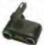
EAD06 Battery saver. Will turn off accessory when battery falls below 11.6v 10A fuse & swivel plug.
